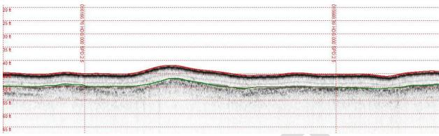
Figure 2: Seismic Line 324 in Site B trending north to south. Green line indicates the digitized consolidated sediment boundary with unconsolidated sediments above.
