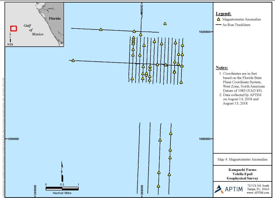
Figure 9. Magnetometer Anomalies Detected during BES Fieldwork (APTIM 2018)
