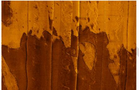
Figure 1: Example of the two identified surface sediment types. Texture 1: high backscatter (upper portion of image). Texture 2: medium intensity backscatter (lower part of image).
