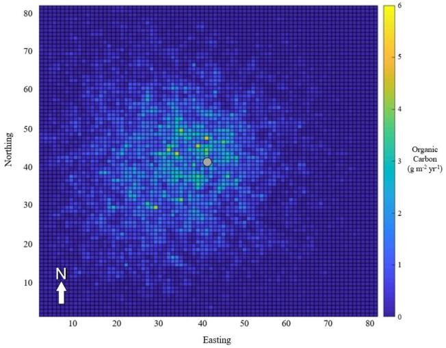
**Figure 3**. Predicted benthic carbon deposition field beneath one net pen with a standing stock biomass of 36,288 kg of Almaco Jack (*Seriola rivoliana*) after five years. Grey circle indicates center position of the net pen. Axes indicate simulation cell numbers and carbon deposition mass is in grams.
