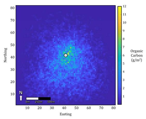
**Figure 4.** Predicted annual benthic carbon deposition field beneath two net pens with a standing stock biomass of 72,560 kg of Almaco Jack (*Seriola rivoliana*). Gray circle indicates center position of the net pen. Axes indicate simulation cell numbers and deposition mass is in grams. The center of the pens is located at (27.056275 N, -83.216743 W). Predicted carbon loading was derived from the 12-month time series relationship based on depositional flux with resuspension.
