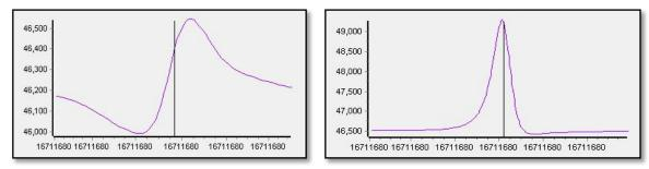
Figure 4: Magnetometer gamma signatures; Left: Dipole anomaly and Right: Monopole anomaly.
